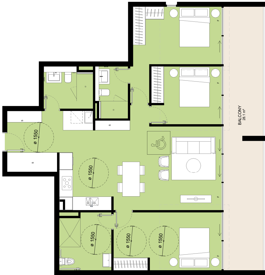
3 LEVEL 14 POST ADAPTABLE UNIT DA3.01 1 : 50
